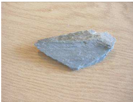
Figure 33: chipping from green Westmoreland slate – the mottled darker appearance of those on houses is a result of weathering and soot.
