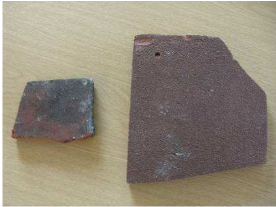
Figure 28: on the left fragment of original Clay tile, on the right an example of the approved Acme sand-face replacement
