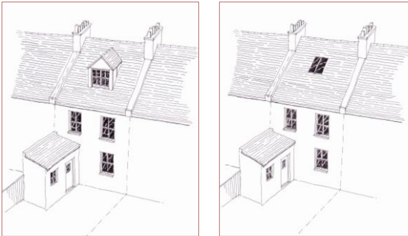
Figure 12: Acceptable designs for dormer window (l) and roof light (r) on buildings with roof slopes not visible from the street
