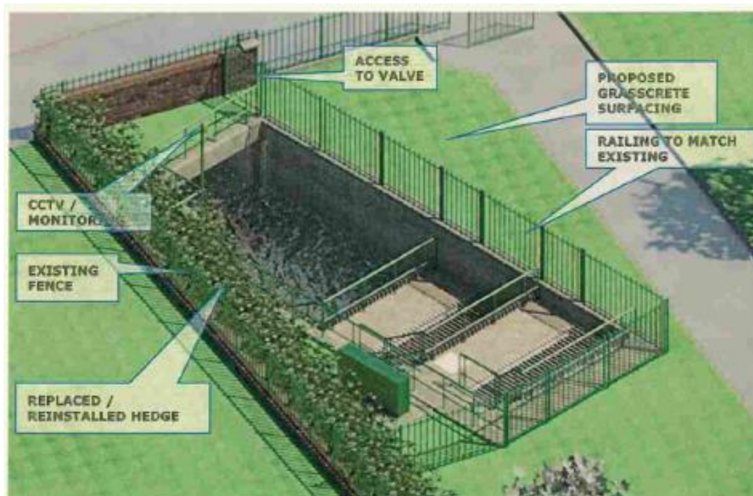
River Quaggy Trash Screen installed in 2018
